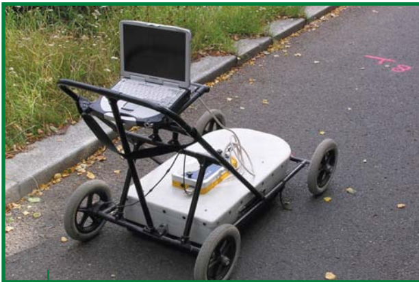
ground-penetrating radar above the sewerage conduit
